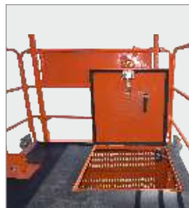
Emergency Exit Gate
